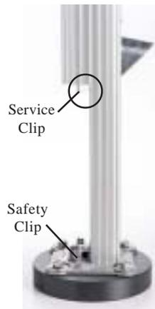
**To Open:** This pedestal has been shipped in the unlock position and is ready to open. Using the outlet cover or FS opening as a hand hold carefully slide the front section of the enclosure up past both the safety clip and the service clip. The top cap of the pedestal moves with this section.
